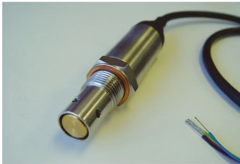
Oil condition monitoring sensor that uses the dielectric constant to determine oil condition. Photo courtesy of Bill Quesnel.
