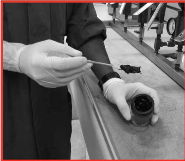
An engine oil subjected to severe overheating
