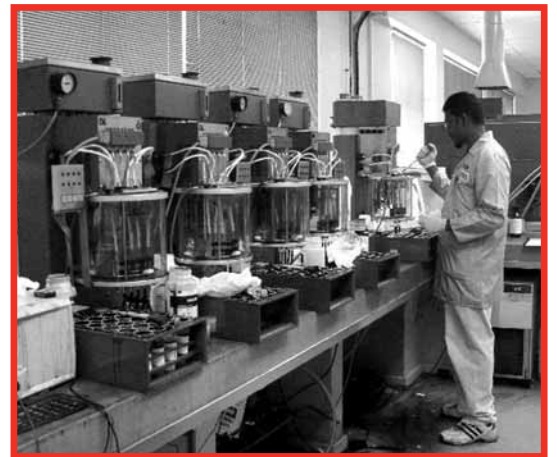
Image 1: Viscosity being measured with a viscometer
