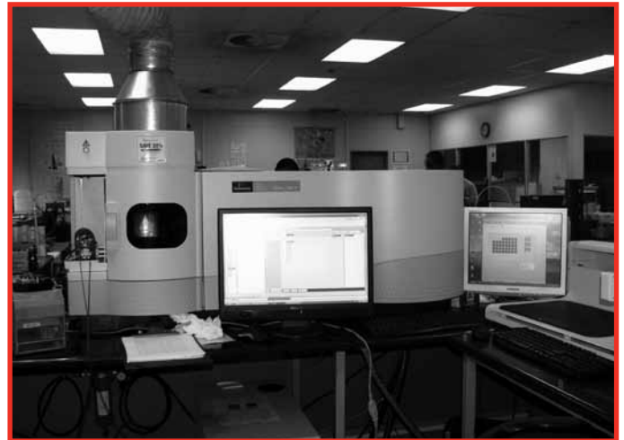
When analysing oil samples, the ICP (inductively coupled plasma) machine provides data such as contamination and wear levels that can be used as part of a holistic diagnosis of the sample
