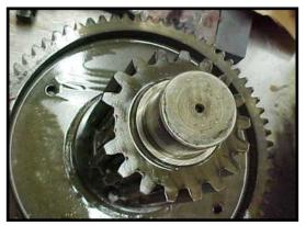
Although the A-Ferr clearly indicated that this unit was going to suffer a catastrophic failure, a maintenance decision was made to do a planned replacement of another assembly line gearbox. The result, the entire plant was shut-down for 12 hours due to this unscheduled failure.
