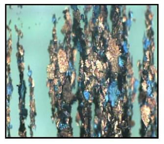
Aside from the analytical ferrography, no other tests indicated any abnormality with this oil sample. The A-Ferr, however, clearly showed severe gear wear, and indicated wear at the gear tooth root. This A-Ferr indicated that a catastrophic failure was imminent.
