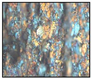
Although the ppm iron level had increased only marginally in this oil sample, the analytical ferrogram clearly indicated catastrophic rolling fatigue wear. The unit was shut-down and inspection revealed a main support bearing that was weeks away from failure.
